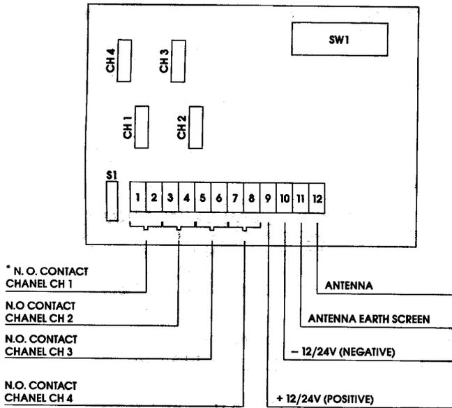
THE CH 1 CHANNEL CORRESPONDS TO THE FIRST BUTTON OF THE TRANSMITTERS.
