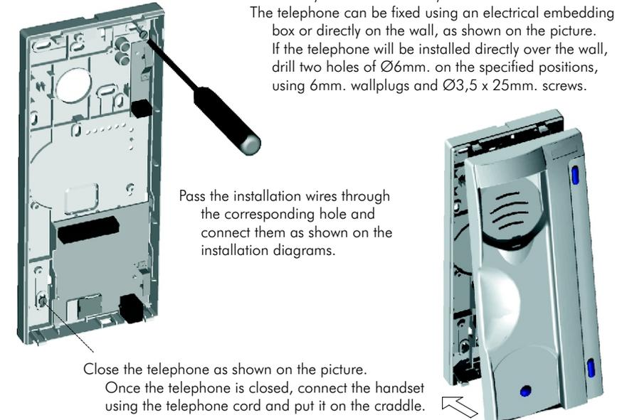
Pass the installation wires through the corresponding hole and connect them as shown on the installation diagrams.
