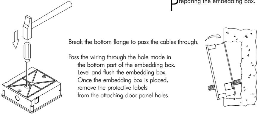
Break the bottom flange to pass the cables through.
