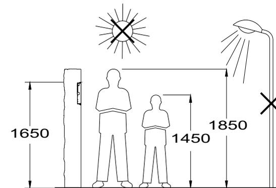
The upper part of the door panel should be placed at 1,65m. height roughly. The hole dimensions are:
