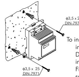
The transformer must be installed in a dry and protected place. It's recommended to protect the transformer by using a thermo-magnetic circuit breaker.
