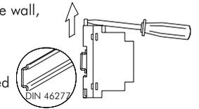
The transformer can be installed on a DIN guide (3 units) simply pressing it. To disassemble the transformer from the DIN guide, use a plain screwdriver to lever the flange as shown on the picture.
