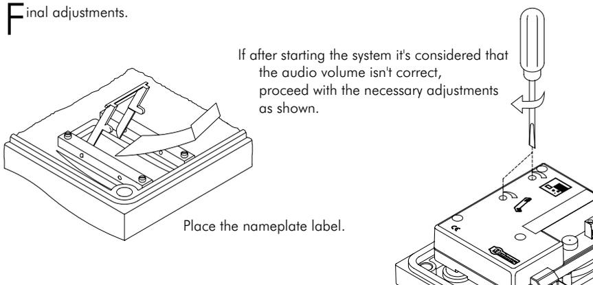
If after starting the system it's considered that the audio volume isn't correct, proceed with the necessary adjustments as shown.
